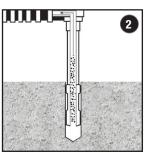
Remove dust and debris from hole during drilling (e.g. dust extractor, hollow bit) or following drilling (e.g. suction, forced air) to extract loose particles created during drilling.
