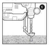
Using the proper drill bit size, drill a hole into the base material to the required depth. The tolerances of the drill bit used should meet the requirements of ANSI standard B212.15
