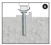
Drive the anchor into the hole until the head of the anchor comes into contact with the fixture. The anchor must be snug after installation. Do not spin the hex socket off the anchor to disengage.
