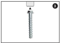
Select a torque wrench or powered impact wrench and do not exceed the maximum torque, Tinst, max or Timpact,max respectively for the selected anchor diameter and embedment. Attach an appropriate sized hex socket/driver to the impact wrench. Mount the screw anchor head into the socket.
